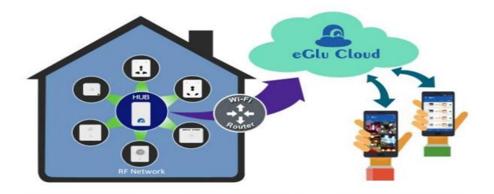
Hub Communicates on low power RF inside the house Hub communicates to eGlu cloud using wifi router
